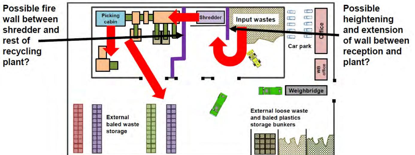
While this would not split the building into 'true' compartments, consideration could also be given to raising the height of and extending the length of the push-wall between waste reception and the shredder to reduce the risk of fire spread (see below on fire walls at bunkers etc).
