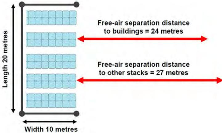
All of the above examples are for general wastes. For plastics and rubber wastes free-air separation distances are wider because of their higher burn temperatures (see graph 2 option 1 above). Use of bunkers is likely the practical option with this type of waste, such as the example of baled plastics shown here. However, an appropriate free air separation distance still needs to be left at the open side of the bunker (from graph 2 using stack dimensions shown).
