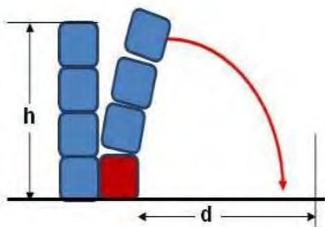
Example of a stack collapse mechanism, assuming a bale at the base of the stack collapses first. The distance any bale, or part of a bale, will 'roll' is dependent on a range of factors making stack collapse too unpredictable to use as a guide to separation distances between stacks
