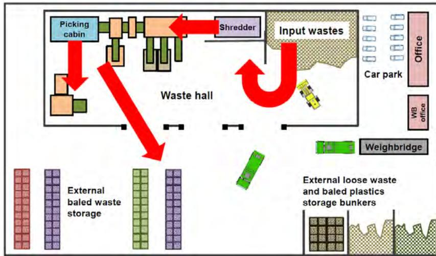
As noted in the section on design above, two of the main fire risks at the illustration recycling plant above are fires in the waste reception area (self-heating, hot and hazardous materials in input wastes etc), which could spread to the recycling plant, and fires in the shredder (gas cylinders, lithium batteries etc), which could also then spread to the rest of the recycling plant.
