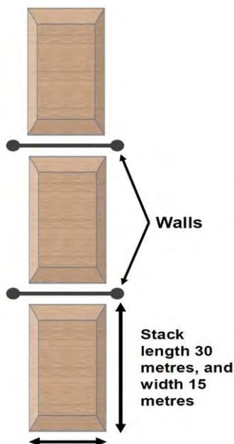
The use of fire walls is not restricted to bale stacks. This example shows a loose stack layout using fire walls to remove the need for free-air separation distances at the width ends of the stack. Assuming good access for fire-fighting is available from both sides stack width is not affected (shown at 15 metres but could be the 20-metre maximum). This type of 'sausage link' layout may be suitable for 'long and thin' waste sites and allows space to be maximised.
