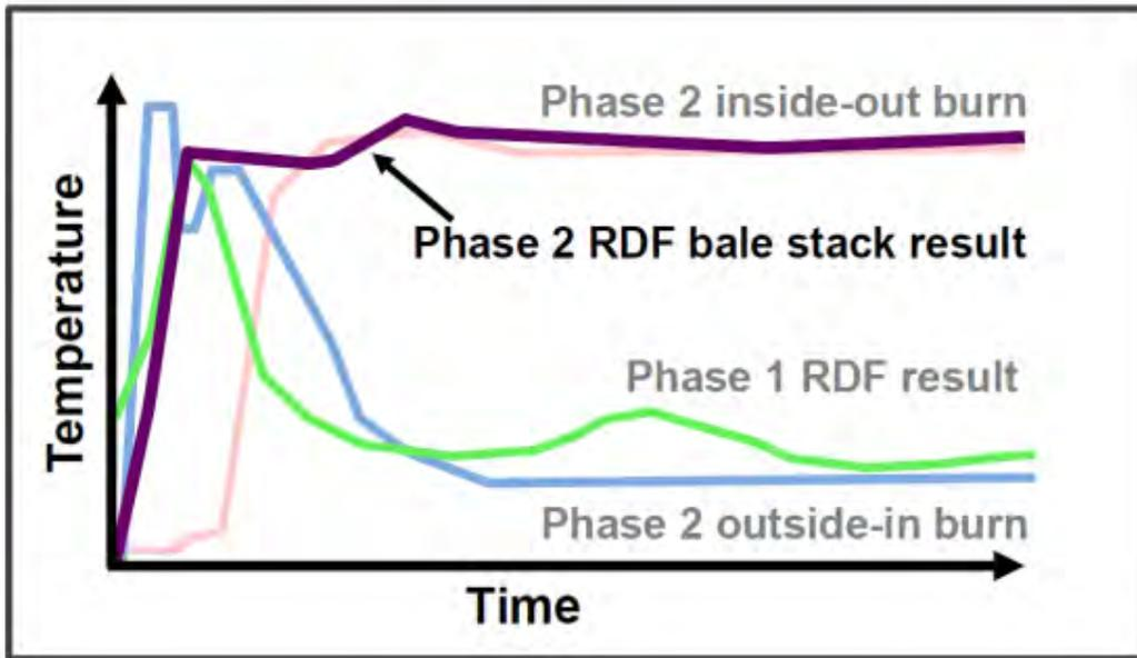
These chimney effects seem to be the likely cause of the energetic and sustained fires with rapid fire spread across baled waste stacks often experienced by the FRS when fighting baled waste stack fires.
