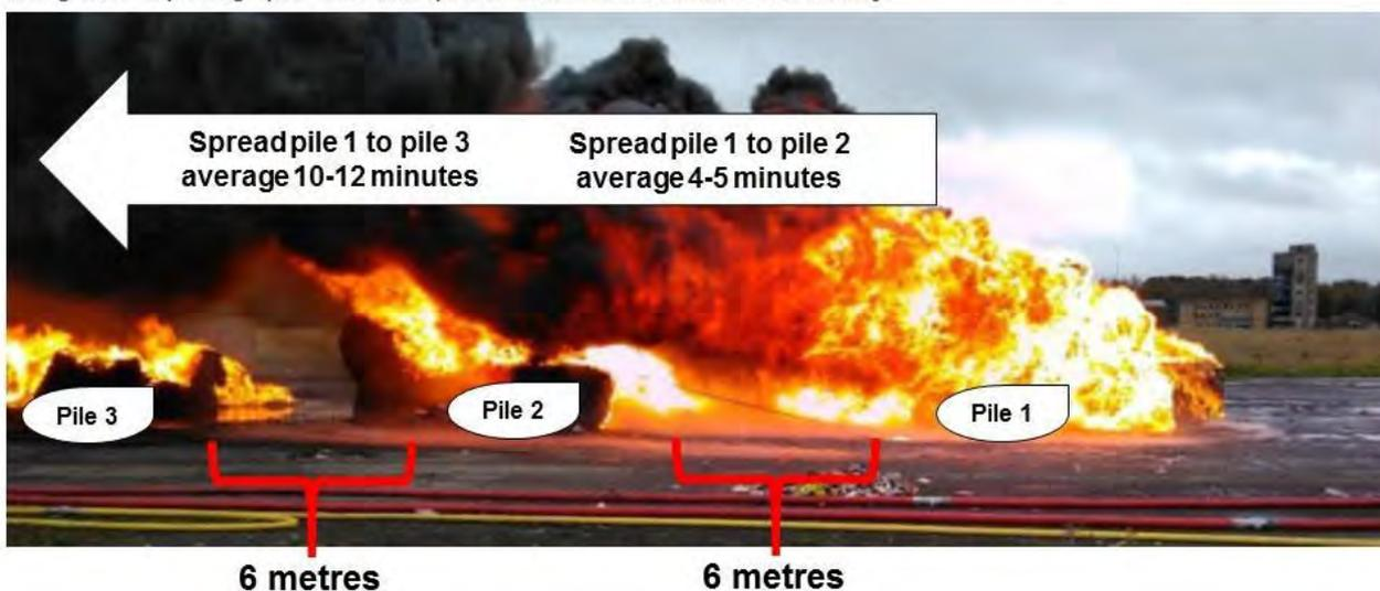
In brief, the results of the WISH fire tests provide the data require to calculate separation distances, and this approach is commonly used by fire engineers as a reliable method'
