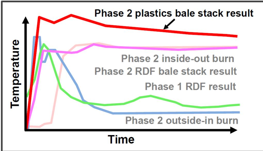
These results largely support FRS experience during fire-fighting of plastic waste bale stacks where temperatures were such that access to fight the fire was, at best, problematic.
