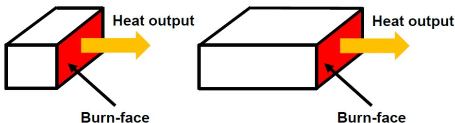
For example, following the waste burn trials calculated separation distances were modelled for two stack volumes ( $450 \text{ m}^3$  and  $750 \text{ m}^3$ ), but with the same burn-face dimensions. The difference between the two sets of separation distances was not significant.
