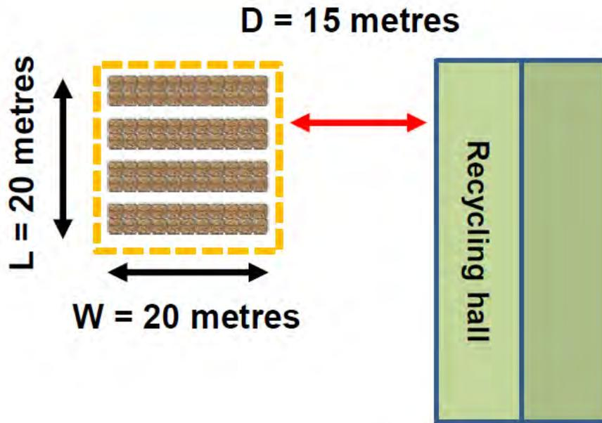
Limited space at this site means the maximum separation distance which can be achieved between recycling building and stack is 15 metres (D in graphic). Using paper/card bales as for example B above, graph 1 purple line gives a maximum stack length of 20 metres (mark 15 metres on the vertical axis of graph 1, draw a horizontal line across to the purple line, and then a vertical line down, giving stack length at some 20 metres). This is an example of a reverse use of the data in graphs 1 and 2.
