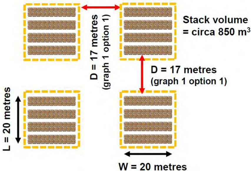
This is similar to above but using paper/card bales (each individual stack of rows of bales demarked by amber dotted line). These are general wastes, so graph 1 applies. Stacks are 20 metres square, giving a separation distance from the brown line in graph 1 of 17 metres each side. Excluding the gaps between bale lines for access, stack volume is circa 850 m<sup>3</sup>, with a total volume across all four stacks of circa 3,400 m<sup>3</sup>.
