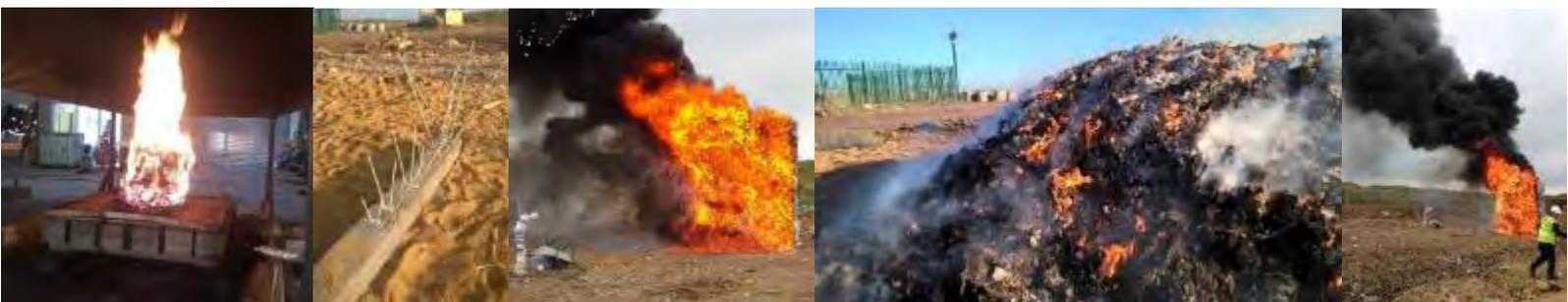
*General views WISH fire tests, from left: Smaller scale laboratory burn tests, the 'porcupine' thermal sensor array used in larger scale stack burns, plastic bales burn test, RDF loose stack burn test, bale burn test general view.*
